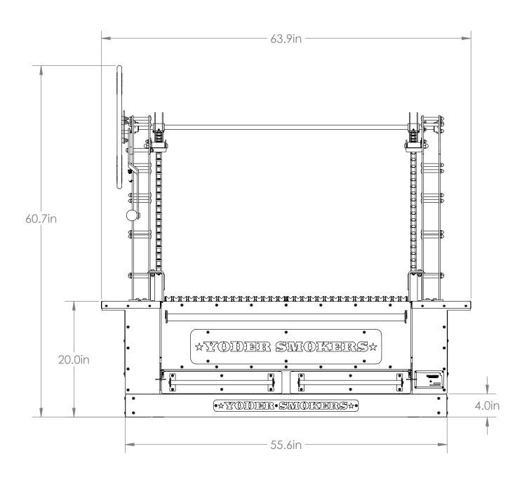
Overall Height: 60.7 in. Overall Depth: 34 in. Overall Length: 63.9 in. Total Weight: 619 lbs.
